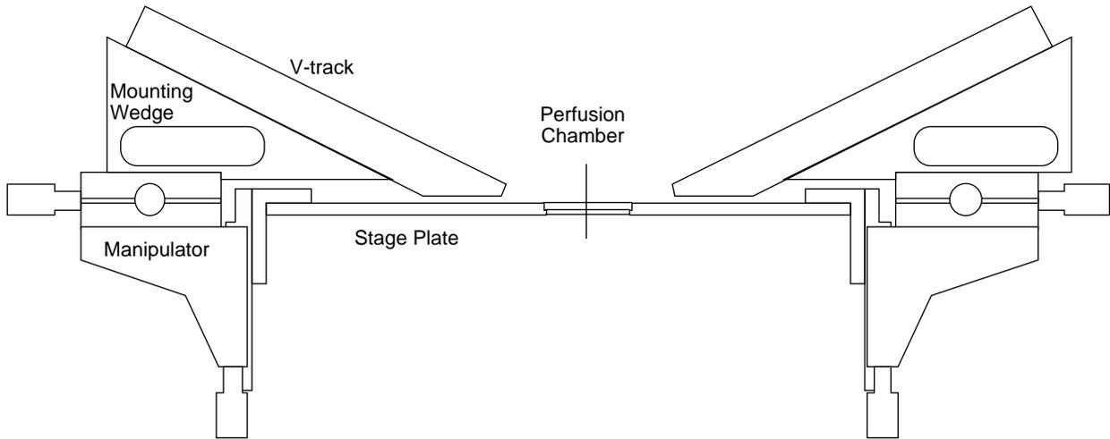
**Figure 1:** Components of the Vestavia Scientific microperfusion system
